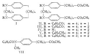
The following outline shows the synthetic route used to make the acids corresponding to the esters of the free diamine IV, the benzamides II, III and the benzyl derivatives V, VI.
